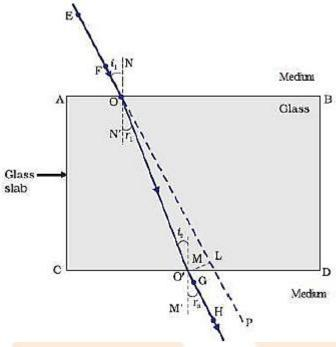
EF is the incident ray and GH is the emergent ray which is parallel to the incident ray.
